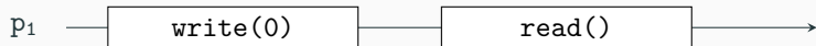
(a) Sequential execution of two operations on a resource R by the process p_1 .
